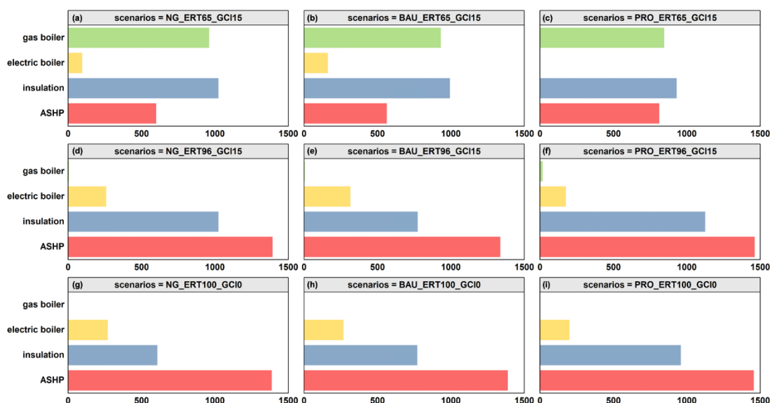
Figure13: Installation numbers of system optimisation measures under different scenarios
